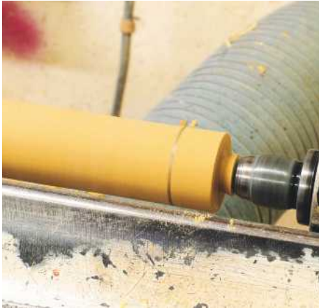
▲ Pic.28 The handle is mounted up between centres. Make it round with the roughing gouge. You can see the amount of waste that Les has allowed at the tailstock end
